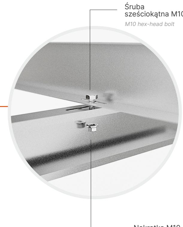
Fasten the cross beams to the main support beams with M10 bolts using slots in the bottom side of the cross beams.
